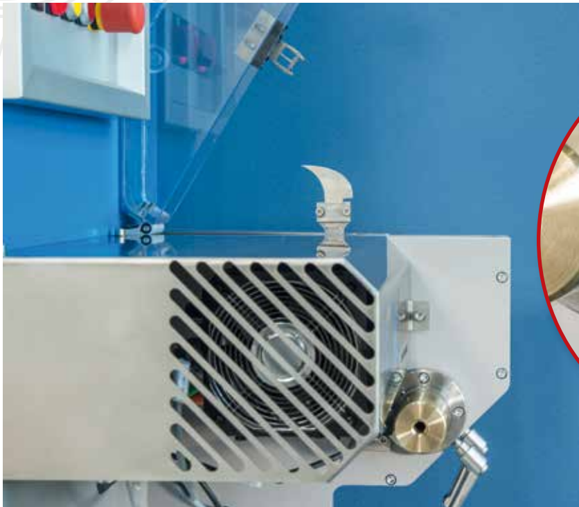
Cutting guide with a tool-free quick-change system
