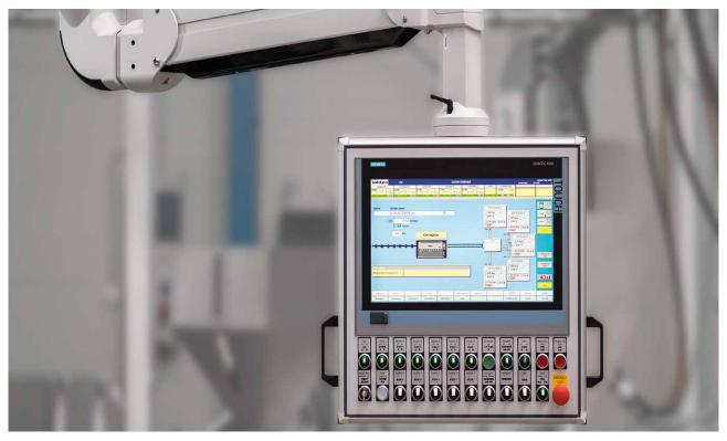
The Bellaform operating interface outputs process data such as temperature curves of the extruder heating or pressure curves in the vacuum tank as a trend curve in real time. Diameter and wall thickness, the distance between the nozzle exit and the calibration or the temperatures in the vacuum tank are recorded. All relevant data are provided in a format that permits further processing or archiving in a superordinate central control.
