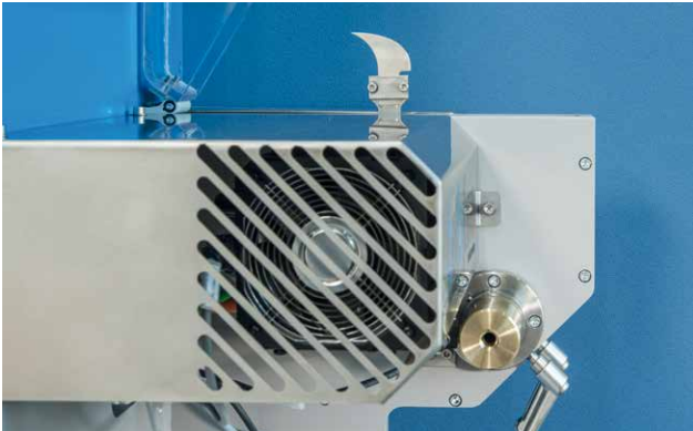
Cutting guidance with quick-change system.
